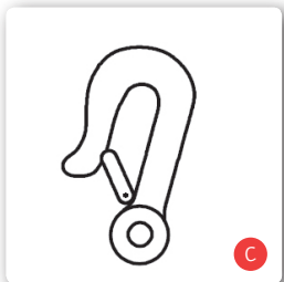
C: Fixing point restraint system
